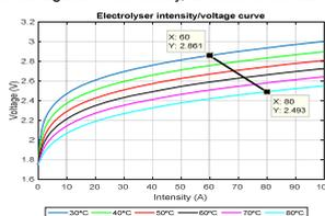
As the operating temperature is increased for the same cell voltage, the intensity crossing it rises. From an energy-based point of view, as the temperature rises hydrogen production becomes more efficient as less electrical power is required
